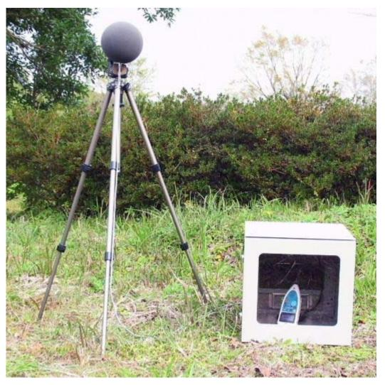
Newly developed material and special waterproofing technology dedicated for the windscreen guarantee easy handling, only coating the microphone.
