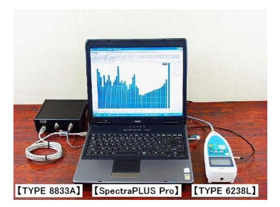
Simultaneous display and analysis for different frequencies are available by using the optional function(scaling/calibration extension) of **NA-0038L(SpectraPLUS pro)**.
