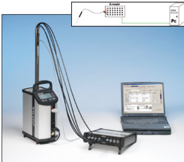
Picture 2: ASM-803 B performing its own measurements in a JOFRA ITC-320 A including an STS reference sensor in channel one all controlled by JOFRACAL.
