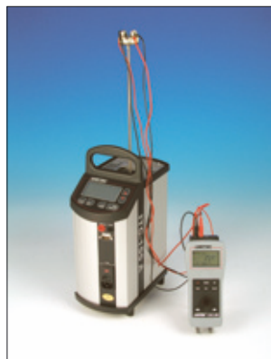
CSC200 as RTD input with an ITC
