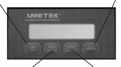
The MENU/ENTER key includes intelligent prompts that guide the user through setup and operation. This key allows the user to specify measuring units, resolution, sensor identification, and coefficients.
