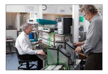
Reference bath calibration is generally regarded as having optimal accuracy. However comparative measurements on a Ø 10mm sensor have shown a maximum deviation of 0,008°C @ 155°C. Compared with a reference bath calibration the calibration result has improved with a factor 3 compared to conventional dry-blocks.
