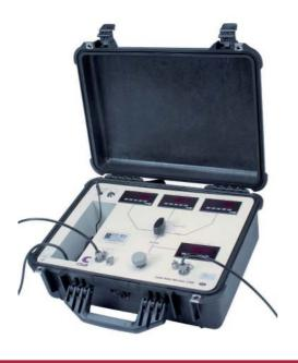
For those who require battery power, any external battery pack of suitable specification can be purchased locally and connected to the +24vdc power inlet. With this design battery packs can be exchanged and recharged without having to remove the LRM from service.
