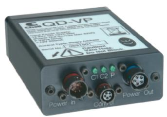
The QD-VP valve module is an accessory to the CANdaq range of acquisition devices. The module contains two solenoid valves designed to control the shuttle of Pressure System ™ ESP pressure scanners. There is also an electrical drive to allow a solenoid valve to control purge gas. The valves are controlled via three address lines, and up to two QD-VP modules may be connected to one QUADdaq. Each valve being independently addressed.
