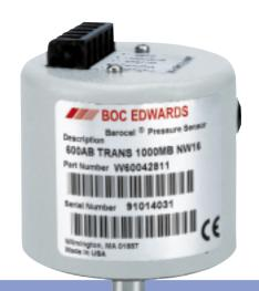
The Model 600 Barocel transducer is an advanced design capacitance manometer which uses patented technology to improve zero stability after temperature excursions or pressure overloads. An integral vacuum reference of all-welded construction contains gettering material to ensure long-term stability.
