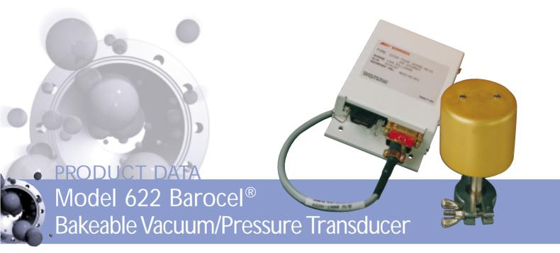
The Model 622 Bakeable Barocel is an adaptation of the field-proven Model 600 vacuum/pressure transducer. The signal conditioning electronic components are separated from the sensor, allowing it to be operated at 200°C as required by some applications. Among these applications are processes involving condensable gases, nuclear processes, and those requiring high temperature sterilization.
