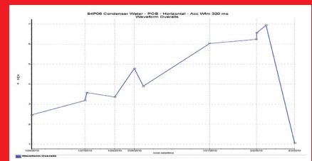
Figure 2. Waveform Overall Amplitude Trend
