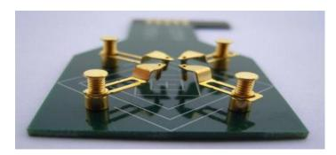
SPCB-3 Spring Clip Sample Mounting Board for samples from 3mm up to 5.5mm thick with square shape and from 5mm up to 20mm on a side:
