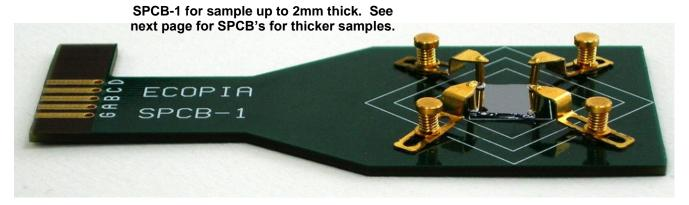
Ecopia offers the following additional models of the SPCB Spring Clip boards. The samples should be square in shape. Construction is of gold plated non-magnetic phosphor-bronze alloy. Contacts applied to the corners of the sample are normally required for good ohmic contact. A complete listing of the available board types is shown on the next page.
