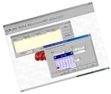
Configuring campaigns is a very intuitive procedure. MicroWin simply provides one Configuration window, where all the basic parameters (such as date and time of campaign start and end, the frequency time, the instrument setup and a descriptive label for each measuring campaign) are set.
