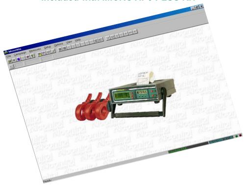
MicroWin allows real-time reading and display of all instrument measures or performing measuring campaigns in two modes: Manual or Automatic. Graphical display includes measuring trends over time, the waveforms and the harmonic spectrum of voltages and currents, etc.
