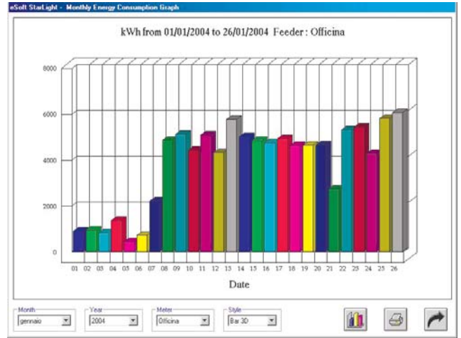
Example of Flexible graphical report. The energy consumption of one department is visible per each single day over the requested period.
