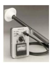
Holaday's HI-1801 provides an easy an inexpensive means for public health agencies and service technicians to check microwave leakage. A durable, compact and portable instrument, the HI-1801 is not susceptible to damage caused by excessive fields.
