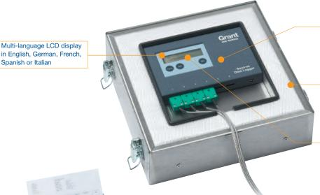
The Squirrel OQ610 data logger can record up to 8 readings per second from all 6 temperature sensors and store 260,000 readings or 8 separate oven runs
