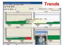
TRENDS Graphical viewing of data collected with preset alarm values and linked pictures as a visual reminder
