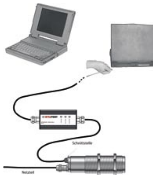
Fig.: Connection example: IKS-Ti - IP 10-USB - Laptop
