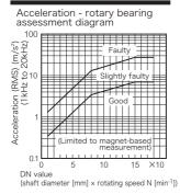
Vibrometer for simple diagnosis use model MK-21 is equipped with an automatic diagnostic function compliant with vibration severity standards (ISO-10816, JIS B 0906), allowing even those operators who have never used a vibrometer to diagnose the status of their facilities.
