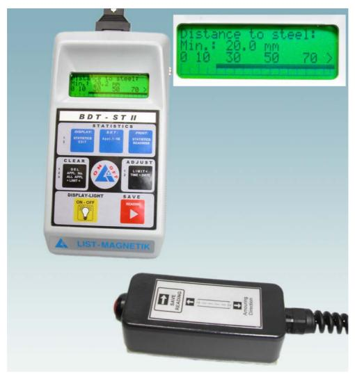
The Concrete Thickness Meters are mainly used in the building trade to determine the thickness of the concrete layer above the armoured steel. This is absolutely necessary to prevent damages of the armoured steel and to avoid expensive restoration.
