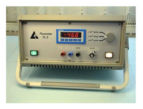
The Fluxmeter FL-3 is an electronic integrator which measures the magnetic flux of all kind of magnetic systems. The main feature of this device is the high sensitivity and a minimum of drift.
