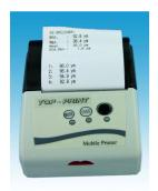
with Bluetooth Interface incl. Charger and Lithium-Ion rechargeable Battery
