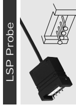
For soft samples Inter-pin distance: 5 mm, pin points \phi 2 ball type, spring pressure: 130 g/pin. RMH116 (MCP-TPLSP)
