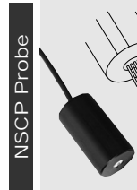
For hard samples Inter-pin distance: 1.0 mm, pin points 0.04R, spring pressure: 250 g/pin. RMJ202 (MCP-NSCP)
