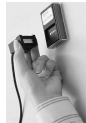
Inspect with a probe checker before measurement.
