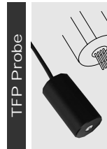
For thin films on glass substrate Inter-pin distance: 1.0 mm, pin points \phi 0.158, spring pressure: 50 g/pin. RMJ217 (MCP-TFP)
