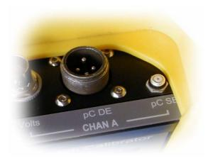
CHARGE OUTPUT is used to simulate the signals from piezoelectric accelerometers. Either Single-ended or Differential signals are available to calibrate and test vibration circuits in machinery monitoring systems. A wide range of charge signals may be produced at constant and varying frequencies.
