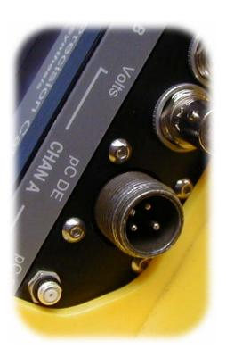
PRECISION CHARGE SIGNALS are produced by the 1500CS. Differential and single-ended signals are available to simulate accelerometers and other charge mode devices.
