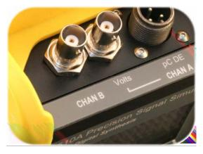
VARIABLE PHASE between the two outputs signals is easily adjusted using the 1510A controls. Use this feature to calibrate balancing and other data acquisition systems.
