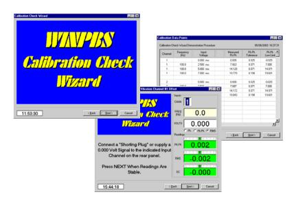
The Calibration Check Wizard provides a quick and easy assessment of the calibration of your PBS-4100R. The program runs on your PBS-4100R system and guides the user through the process of connecting precision signals to each of the vibration input channels. At the conclusion of the test, a table is displayed indicating which channels are within factory tolerances and which are not.
