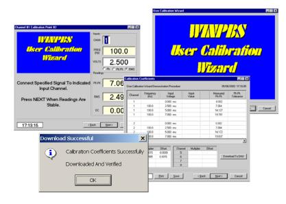
The User Calibration Wizard guides the user thru the process of re-calibrating all of the PBS-4100R input channels using different amplitude and frequency signals. Each channel is checked for offset and accuracy at several levels throughout the measurement range. At the conclusion, a table summarizes all of the measurements, and the internal PBS-4100R system calibration factors are updated.
