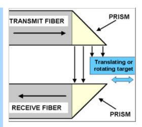
The fiber optic probe directs a "curtain" of light past the measurement target edge to an opposing receive fiber bundle. As the target moves within this "curtain", the intensity of light received changes proportionally with the edge position. The MTI-2000 Controller precisely converts this signal to an edge position or vibration amplitude.
