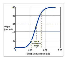
This plot shows a typical response curve for the Fotonic Edge probe that relates the amount of light received to the radial displacement of the edge under measurement. With the Fotonic Edge probe, you can make measurement as sensitive as  $0.1 \, \mu in./mV(2.5 \, nm/mV)$  over a linear range of approximately  $0.004 \, in. \, (0.1 \, mm)$ .
