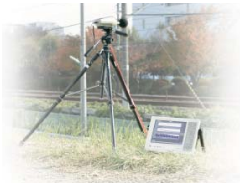
Outdoor noise analysis using the CF-7200 and an LA Series Sound Level Meter
