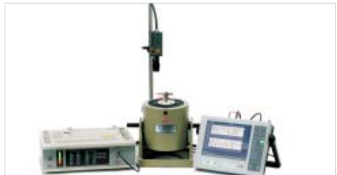
Analysis of micro-object using a LV Series Laser Doppler Vibration Meter and a magnetoelectric shaker
