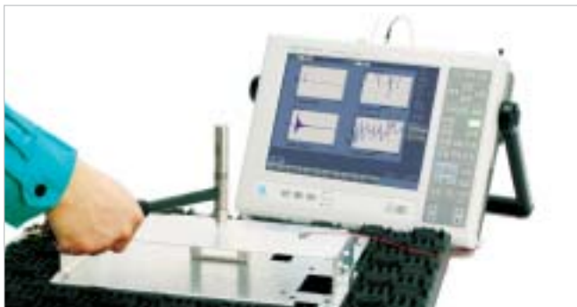
Hammering measurement with the CF-7200, GK-3100 Impulse-force Hammer and an NP Series Accelerometer
