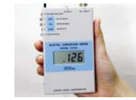
Displacement display 0.126 mm (126 \mu m )
