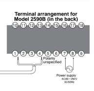
Vibro Converter (w/ built-in detector)
