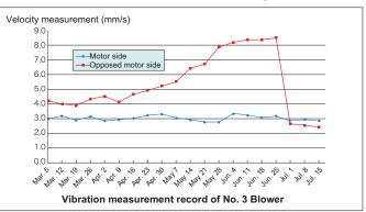
Similarity comparison: This method compares vibration values of machines of the same type and judges a machine of the higher vibration value (indicating the machine is abnormal).
