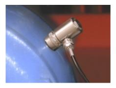
Special transducers for shock pulses and vibration assure accurate measurements. On measuring points that are unaccessible during normal operation, the transducers are permanently installed and connected to measuring terminals.
