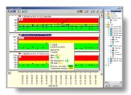
The Condmaster®Pro graphics functions make it easy to follow condition development. Comparing the diagrams for different measured quantities pinpoints the cause of faults, allows estimates regarding the urgency of repairs, and thus efficient maintenance during planned machine stops.
