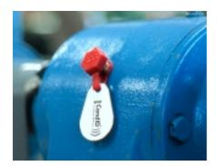
The latest labour-saving technique: contact-free ID tags load the instrument with all measuring point data and also save the latest measuring results. Aerials for RF transponders are built into the Logger and Expert versions of the T30.
