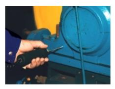
Speed data are necessary for condition evaluation, and monitoring the machine temperature often supplies valuable information. T30 uses temperature probes for solids and liquids. Speed is measured by contact, or optically from a safe distance.
