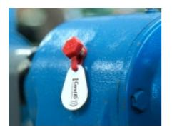
The latest labour-saving technique: contact-free ID tags load the instrument with all measuring point data and also save the latest measuring results. Aerials for RF transponders are built into the Logger and Expert versions of the A30.
