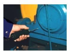
Speed data are necessary for condition evaluation, and monitoring the machine temperature often supplies valuable information. A30 uses temperature probes for solids and liquids. Speed is measured by contact, or optically from a safe distance.
