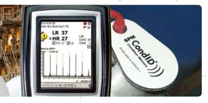
Contact free measuring point identification with SPM's patented Condition Memory.
