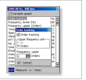
Order tracking is an optional Leonova function primarily used for vibration analysis on variable speed machines. The method uses multiples of rotational speed (orders), rather than absolute frequency (Hz). The number of orders to be shown is input by the user. Leonova will then automatically set the sampling frequency to an exact multiple of the measured rpm. Order tracking will also minimise the risk of smearing when using FFT averaging.
