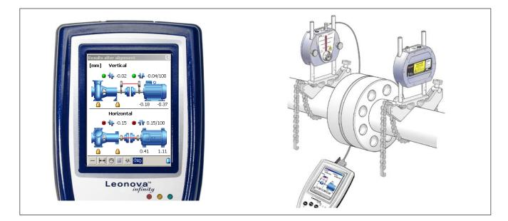
Shaft Alignment is an optional Leonova<sup>™</sup> function for quick and easy shaft alignment, with either limited or unlimited use. In case of limited use, credits are deducted for each alignment assignment. The function is user-friendly and easy to learn.
