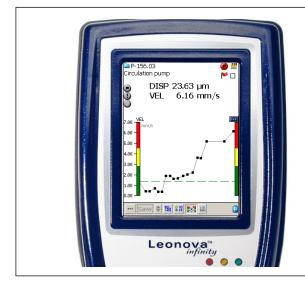
Broad band vibration measurement is the most widely used and cost-efficient method for the diagnosis of general machine condition.
