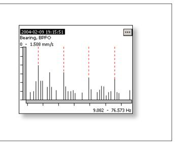
FFT Spectrum with Symptoms is a vibration analysis function offered with Leonova, for either limited or unlimited use. It is a reduced form of EVAM (Evaluated Vibration Analysis Method), lacking the statistical evaluation by means of criteria and possibility to display and save time signal (option).
