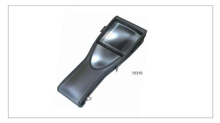
Protective cover 15310 is an optional accessory for the hand-held machine condition analyser Leonova<sup>™</sup> Infinity. The cover, made of foamed polyester fabric, protects the instrument against shocks, splashes and dirt (IP64). The transparent plastic window makes Leonova easy to operate via the keypad and can be opened to facilitate the use of the touch screen. The cover is provided with holders for wrist strap and stylus.
