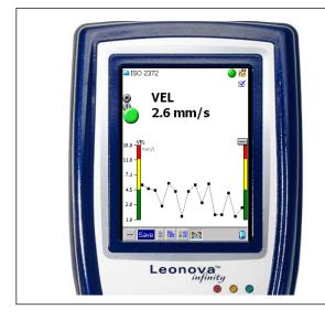
Broad band vibration measurement is the most widely used and cost-efficient method for the diagnosis of general machine condition. There are two ISO recommendations concerning this type of machine condition monitoring, the much used ISO 2372 and the more recent ISO 10816, which is a ongoing replacement of the older standard.
