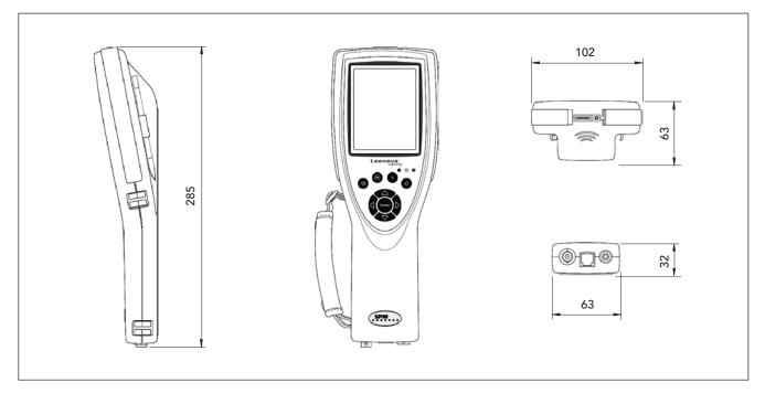
Leonova Infinity is a multi-function, hand-held data logger. The instrument is operated via keypad and touchscreen. Basic data for the measurement set-up can be input manually or downloaded from Condmaster®Nova.
