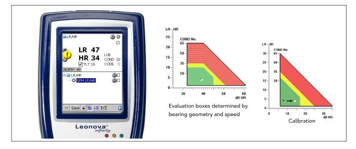
The LR/HR method was developed from the original Shock Pulse Method for condition diagnosis of rolling element bearings. It allows a precision analysis of oil film condition in the rolling interface and contains calculation models for finding the optimal lubricant. Poor lubrication is the root cause of most bearing failures.
