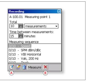
Recording is an optional Leonova function with unlimited use. It allows the user to measure simultaneously with up to three different transducers and record measuring results for as long as the battery charge will last. Thus, 'Recording' is an analysis tool that can show the interaction of various condition parameters over time.
