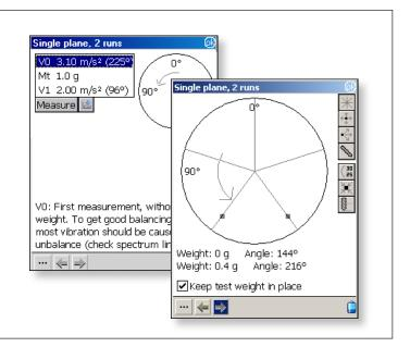
Single and dual plane balancing are optional Leonova functions with either limited or unlimited use. In case of limited use, credits are deducted for each vibration measurement.
