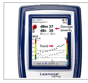
The purpose of 'SPM Spectrum' is to verify the source of high shock pulse readings. Shocks generated by damaged bearings will typically have an occurrence pattern matching the ball pass frequency over the rotating race. Shocks from e. g. damaged gears have different patterns, while random shocks from disturbance sources have none.
