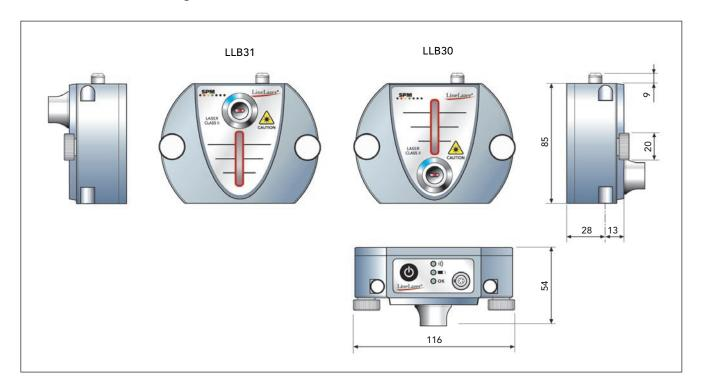
LineLazer<sup>III</sup> LLB30 and LLB31 are two detector/transmitter units for shaft alignment with the multi-function datalogger Leonova<sup>III</sup>. The detectors are identical with exception of the position of laser diode and sensor.
