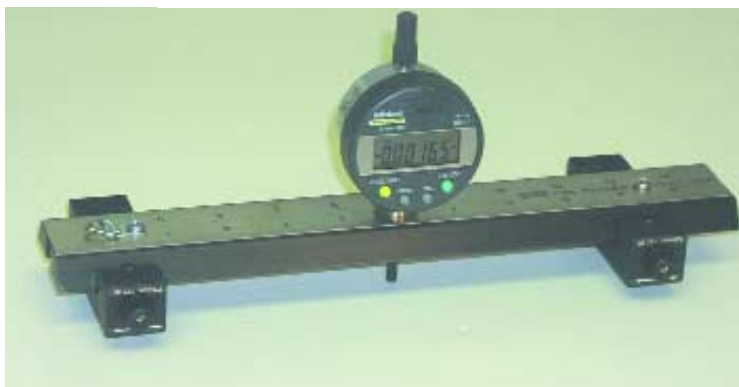
Figure 5. Three-point roll wave gauge with digital readout
