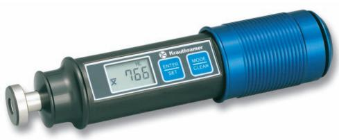
In the setup or configuration mode, you can select different settings, in this case e.g. the required hardness scale (SCAL), or a material group (MAt). Other setting options: Single/Average, conversion according to DIN 50150, ASTM E 140, or instrument-specific conversion.
