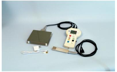
The Trek Model 159HH Hand-Held Charged Plate Monitor is a compact, highly accurate hand-held instrument that can be used to measure air ionization system performance characteristics such as electrostatic decay and ion balance. Its user-friendly operation makes it suitable for frequent use in gathering data and inspecting systems in the workshop or on the production floor.
