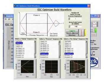
The Trek Model 640 Electrostatic Chuck Optimizer system allows Scientists and Engineers the freedom to experiment and optimize the waveforms and voltages required by an electrostatic chuck/clamp. The Model 640 system can be used to research, facilitate, and discover the exact waveform to minimize the de-clamp time and the precise voltage amplitude to maximize clamp force and maintain optimum wafer processing for your particular ESC operation.
