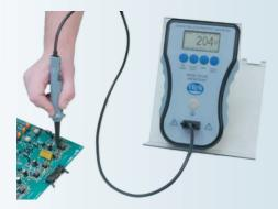
Trek's Model 821HH Infinitron<sup>®</sup> Hand-Held Electrostatic Voltmeter represents the next generation of contacting precision surface voltage measuring instruments, providing input characteristics far beyond the limits of any currently available hand-held voltmeter product.
