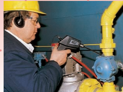
Ultraprobe 100 testing pump valve leaks
