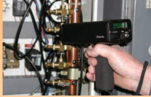
Detect air leaks
