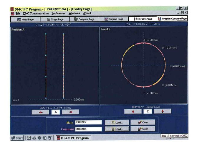
The OVALITY page is intended for cylinder liner ovality measurements only. Page <u>F5</u> will display "OVALITY DIAGRAM". This is automatically changed by the DI-5C when selecting 'Crankshaft measurement' or 'Ovality measurement' during set-up of the DI-5C.
