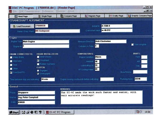
The HEAD page (F1) allows you to register Ship / Plant name, and other basic information such as engine type and number. If measuring a "Vee" engine, check the Vee engine box. Then the word "CYL" will be replaced by "WEB" in the program. You may write down additional information in the "Remarks" box at the bottom of the screen. To printout the page, go to "File – Print Document", check the requested page(s) and press OK.
