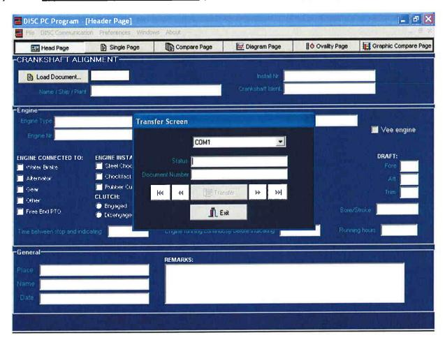
Select the COM-Port on which the instrument is connected in the Transfer screen.
