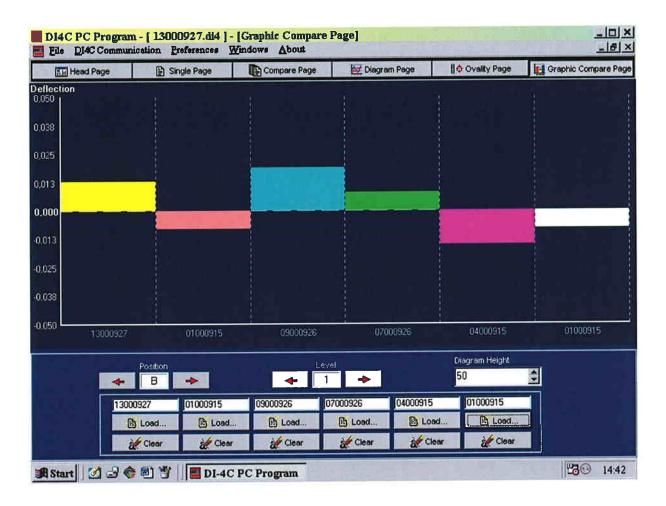
Pressing the <u>F6</u> key brings up the GRAPHIC page, where up to six different document readings may be displayed and compared on-screen, to show trends and to ease decision of necessary actions. It can also be found under the 'Windows' menu.
