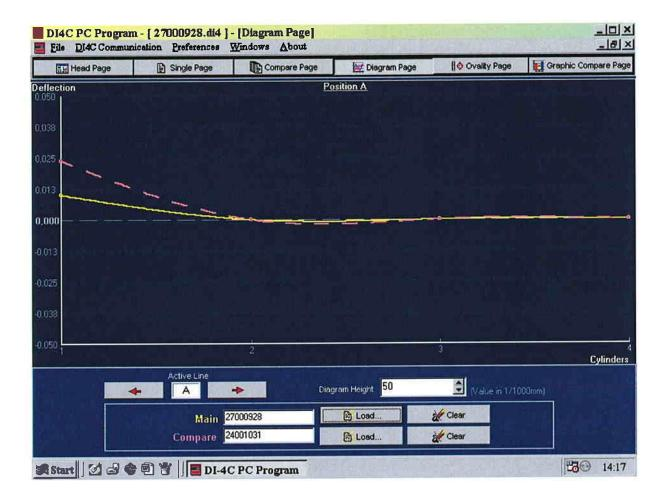
The DIAGRAM page ( $\underline{F4}$ ) produces a +/- deflection curve for each position of the crank/cylinders, e. g. all position "A" crank readings for each cylinder, maximum 24 cylinders per document in a crankshaft measurement.
