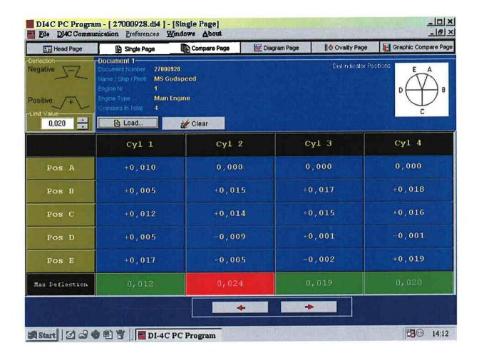
The SINGLE page (F2) shows the DI-5C readings in sequential cylinder order. For Crankshaft deflection measurement the Header is Cyl 1, Cyl 2, Cyl 3 etc. (cylinder). If the "Vee engine" box on the Head page is checked, "Cyl" will be exchanged to "Web". If the document is a cylinder liner Ovality measurement the Header will state Lev 1, Lev 2 etc. (level). The top left picture illustrates the meaning of positive and negative deflection.
